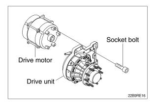
4 Loosen six mounting bolts on the truck frame and carefully take out the drive unit.
