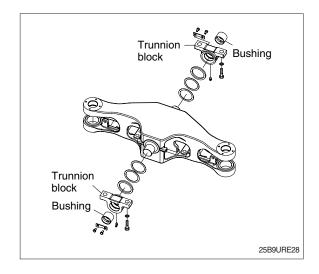
(2) Install the trunnion block so that the clearance is under 0.5mm when the trunnion block is pushed fully to the rear. Tightening torque of mounting bolt for trunnion block. Apply loctite #277.
