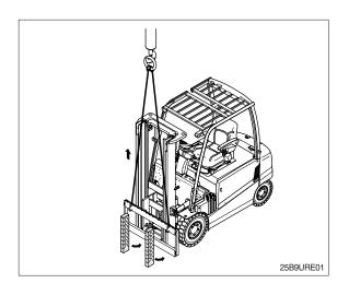
While supporting lift chains, remove the split pins and nuts from anchor pins of stationary upright.
